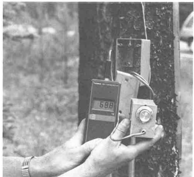
FIGURE 9 Electronic thermometer and switching box, Site D2-92-45.2.
