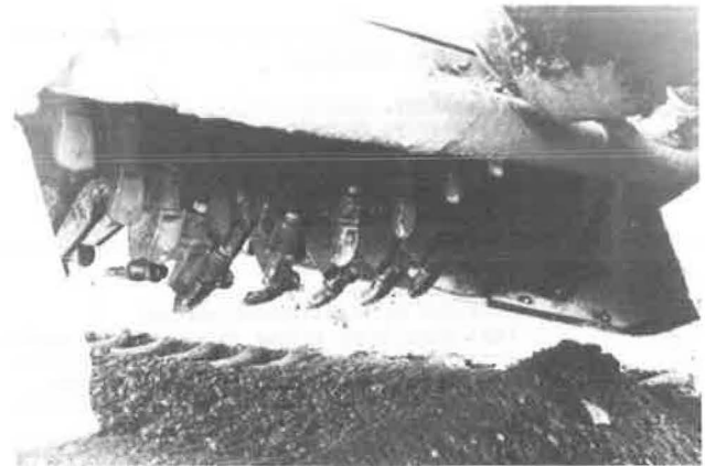
FIGURE 4 Underside of rotomill showing cutting teeth.
