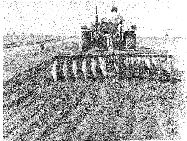
FIGURE 23 Disc harrows for pulverization of soil clods.
