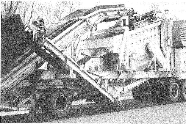
FIGURE 2 Screening and crushing unit.
