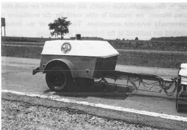
FIGURE 1 Dynalect positioned at a typical crack in a jointed pavement.
