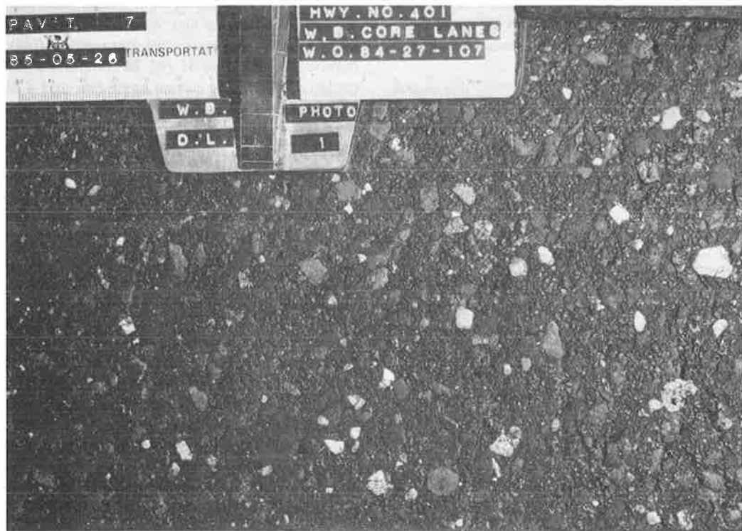
FIGURE 4 Close-up of wheelpath of driving lane of Section 7 (steel slag coarse aggregate, steel slag screenings fine aggregate) after 11 years of service; friction is excellent, and macro- and microtexture are good.
