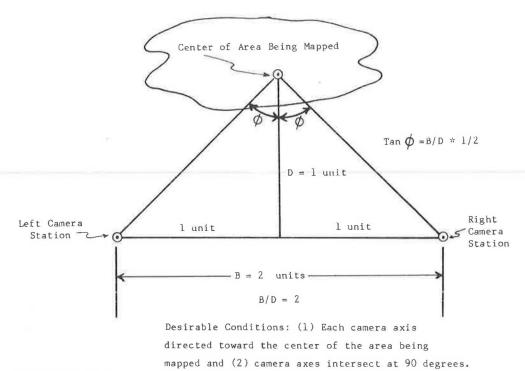
FIGURE 1 Optimum camera configuration.
