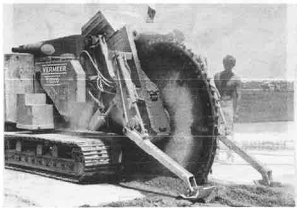
FIGURE 3 Concrete cutting wheel.
