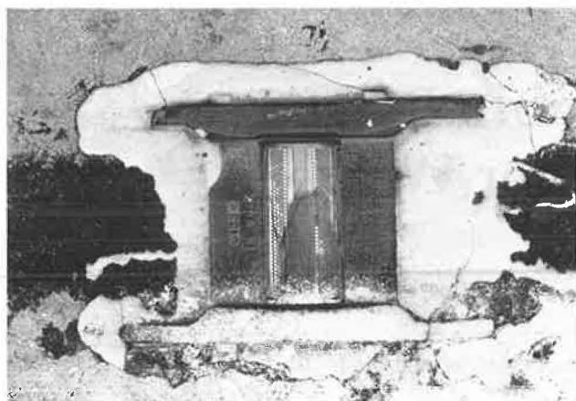
FIGURE 2 Cracked reflector with top delamination.
