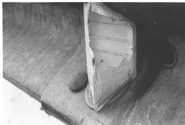
FIGURE 1 Stimsonite acrylic guiderail delineator with broken casing and face.
