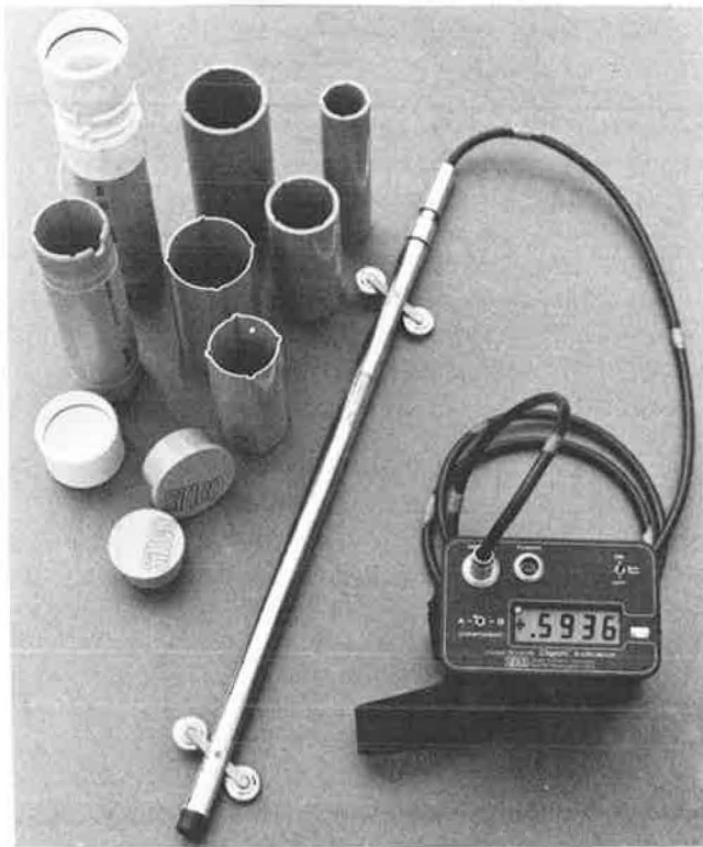
FIGURE 6 Digitilt inclinometer, manual readout, inclinometer casing, and couplings.
