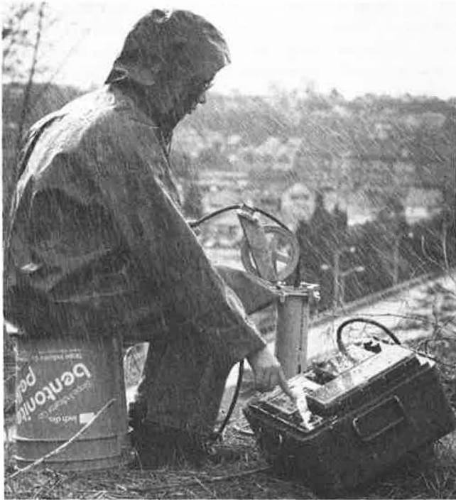
FIGURE 7 Digitilt inclinometer in use with recorder, processor, and printer (RPP).
