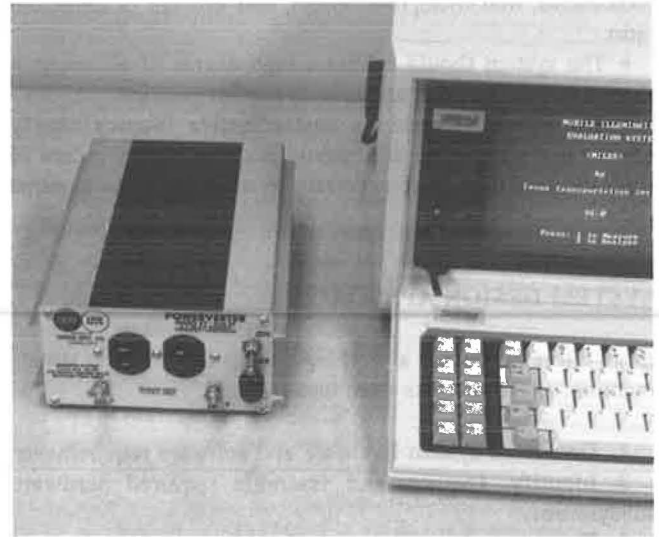
FIGURE 4 System power inverter.
