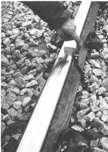
FIGURE 6 Reprofiled rail with gage.
