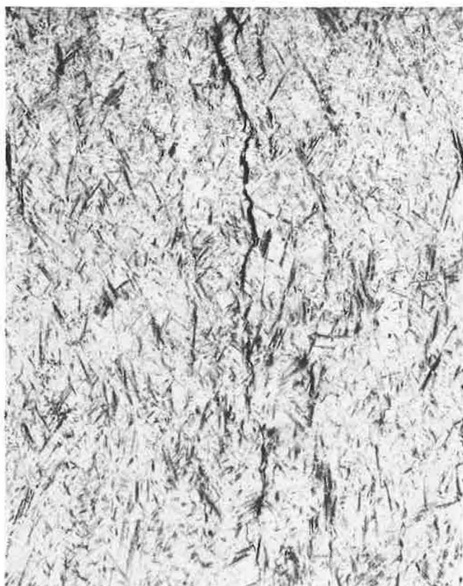
FIGURE 21 Photomicrograph of transverse cracks associated with a brittle martensitic weld metal.
