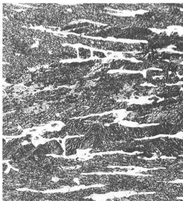
FIGURE 18 Photomicrograph of undiluted Cr/Mn weld metal.
