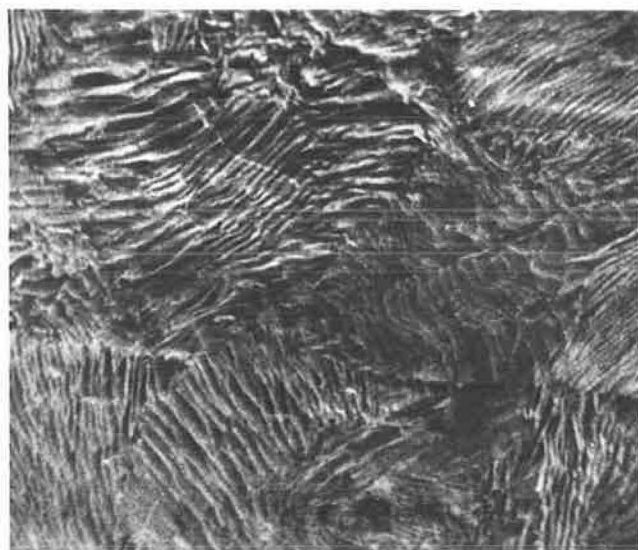
FIGURE 9 Fine lamellar pearlite structure ( \times 4,745 ).
