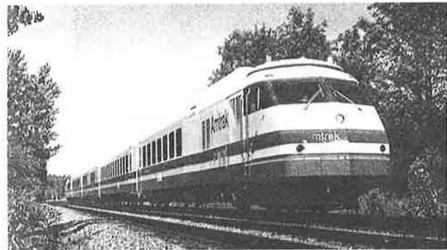
FIGURE 23 Gas-turbine trainset Turboliner (United States): maximum speed 200 km/h, rated turbine power 1700 kW.
