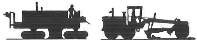
1 Dynaplane rips and pulverizes the pavement, adds asphalt binding agent, and thoroughly mixes in a single pass.
