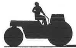
3 Roller compacts material.
