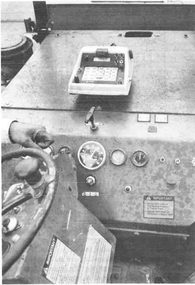
FIGURE 2 Operator view of microprocessor mounted on compactor.
