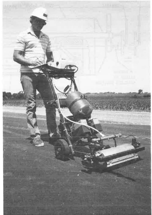
FIGURE 3 DOR system mounted on a two-wheeled cart. Cart may or may not be motorized.
