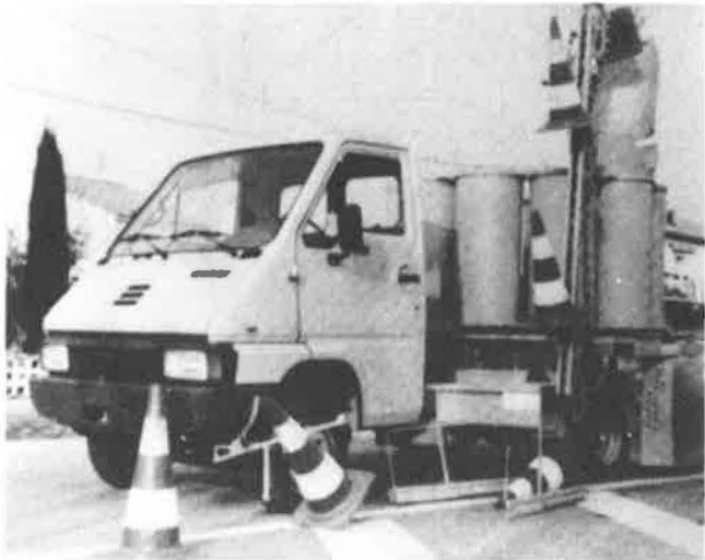
FIGURE 2 Experimental cone dispenser picking up cones.
