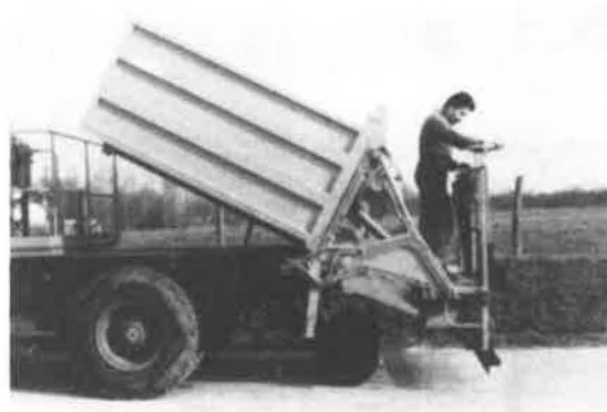
FIGURE 9 The 4-m 3 tipper with built-in tailboard spreader.
