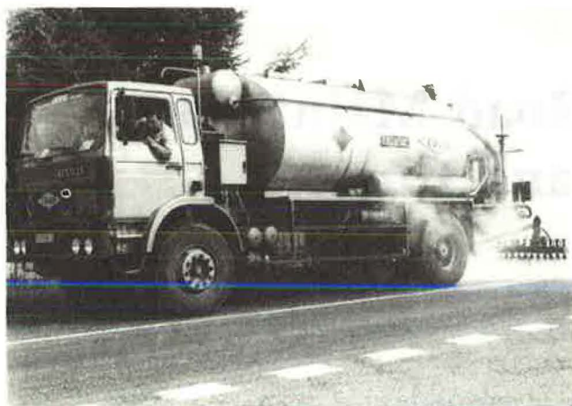
FIGURE 1 Modern asphalt distributor, for all asphalt binders, outfitted with electronic drives to provide uniform distribution of material.
