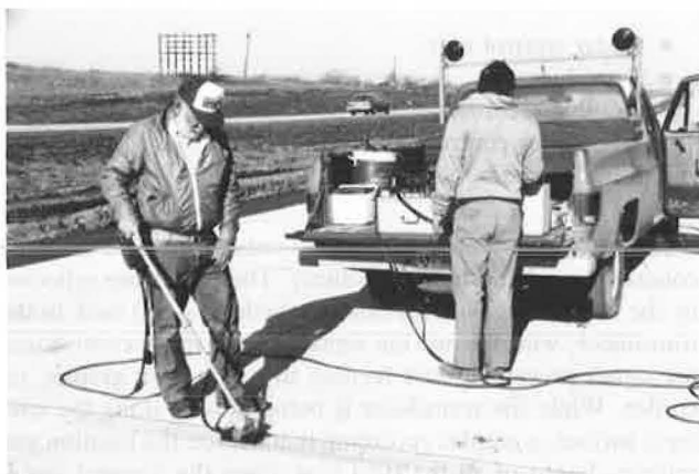
FIGURE 2 Radar test setup at transverse joint.
