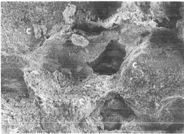
FIGURE 10 Cored cemented coquina highway base course, 59 percent carbonates ( \times 218 ).
