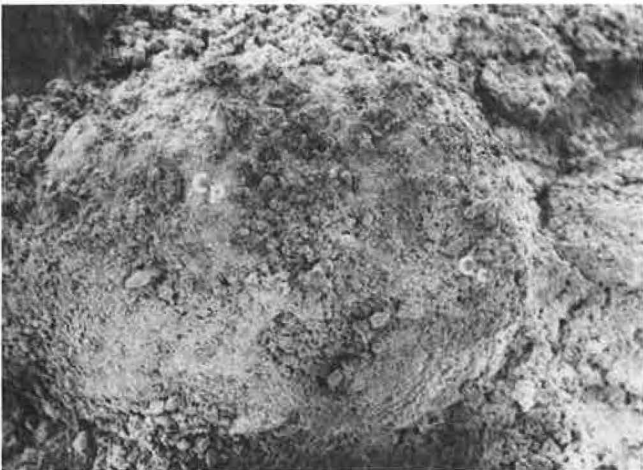
FIGURE 6 Sand mix, 100 percent carbonates, 1 percent \text{Ca}(\text{OH})_2 , 14-day soak ( \times 143 ).
