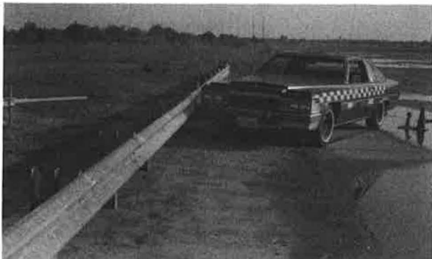
FIGURE 15 Modified guard fence No. 3 and car before and after Crash Test 3.
