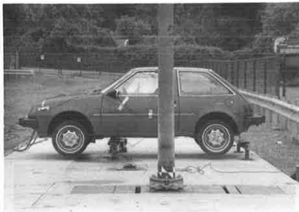
FIGURE 4 Side impact vehicle guidance system.
