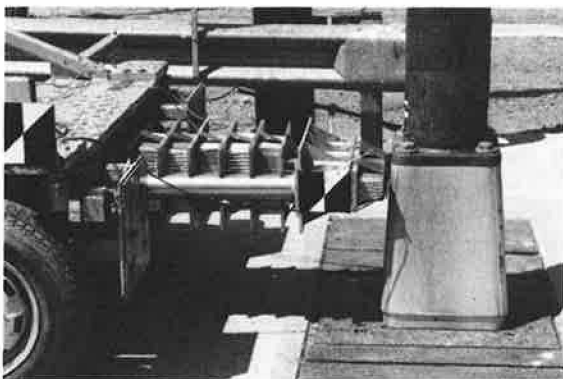
FIGURE 2 Frontal impact bogie test vehicle.
