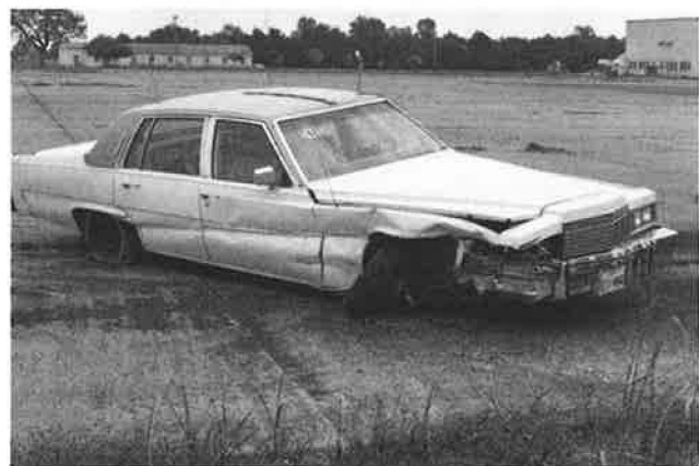
FIGURE 15 Vehicle damage after Test 3.
