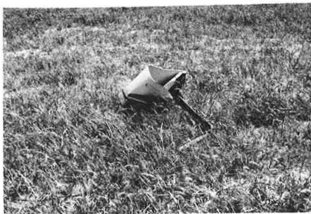
FIGURE 9 Damage to mailbox system, Test 4.
