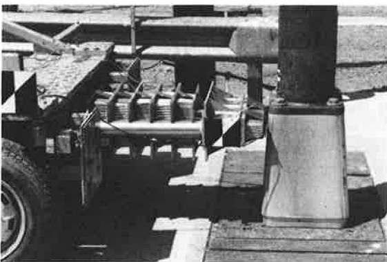
FIGURE 2 Frontal impact bogie test vehicle.
