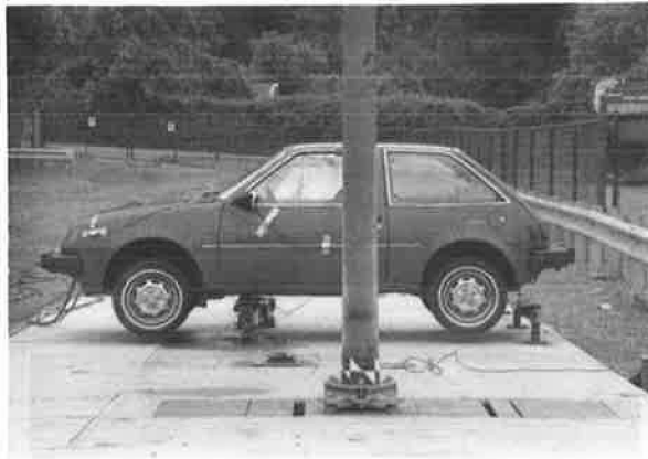
FIGURE 4 Side impact vehicle guidance system.
