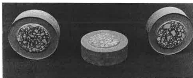
FIGURE 5 Prepared concrete specimens.
