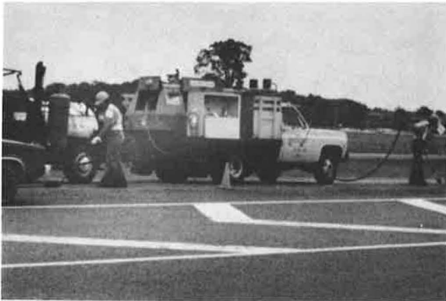
FIGURE 10 Standard ministry equipment train for in-house rout-and-seal operations.
