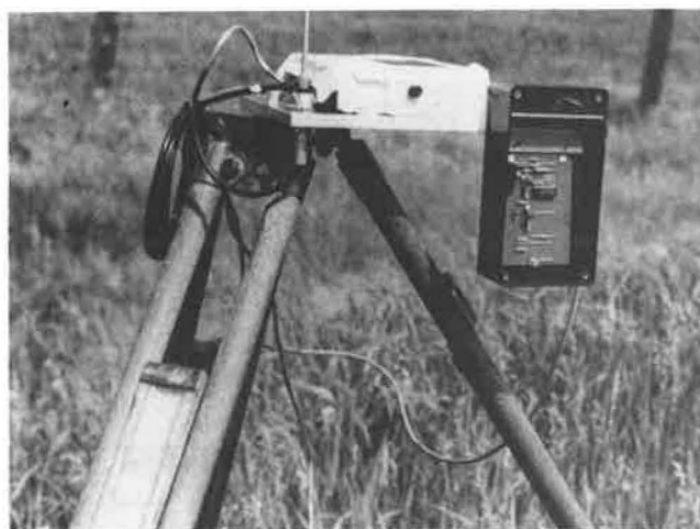
FIGURE 4 Axle detector and transmitter assembly.
