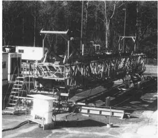
FIGURE 1 Accelerated Loading Facility machine at the FHWA Pavement Testing Facility.
