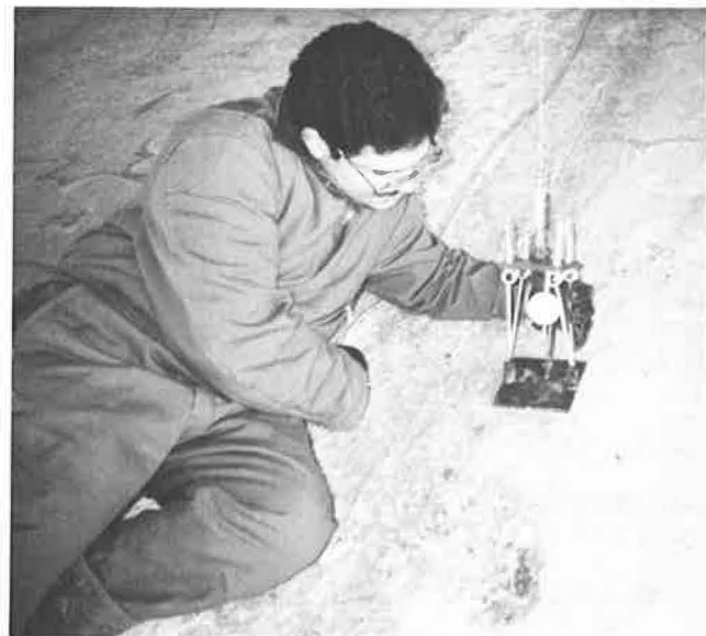
FIGURE 14 Typical deflection measuring device. Top , schematic and bottom , view of installed device.
