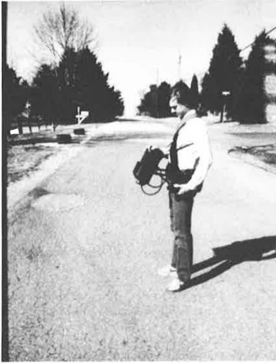
FIGURE 3 Infrared scanner mounted on portable body harness.
