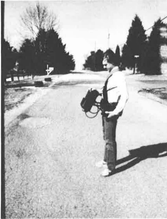
FIGURE 3 Infrared scanner mounted on portable body harness.
