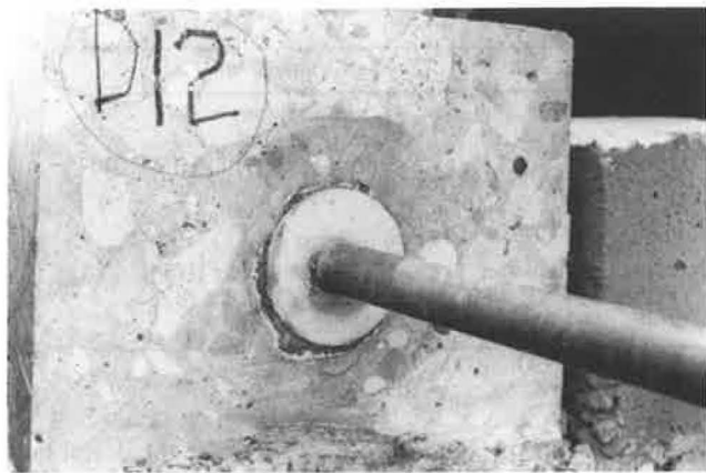
FIGURE 2 Photo of grout retention disk installed on test specimen.
