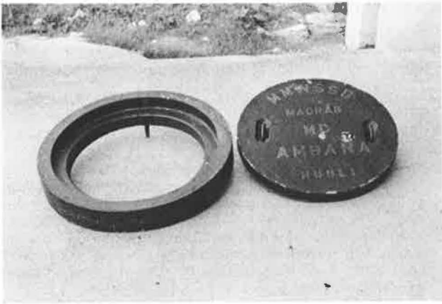
FIGURE 3 Fiber reinforced concrete manhole cover and frame developed at SERC, Madras.
