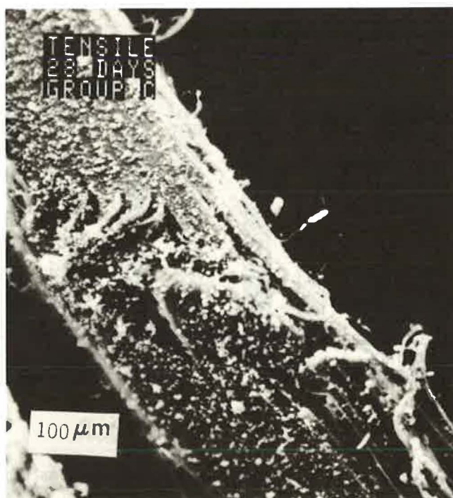
FIGURE 4 Scanning electron micrograph of fiber surface morphology of a failed fiber from the splitting tensile test of treatment group C (28-day cure).
