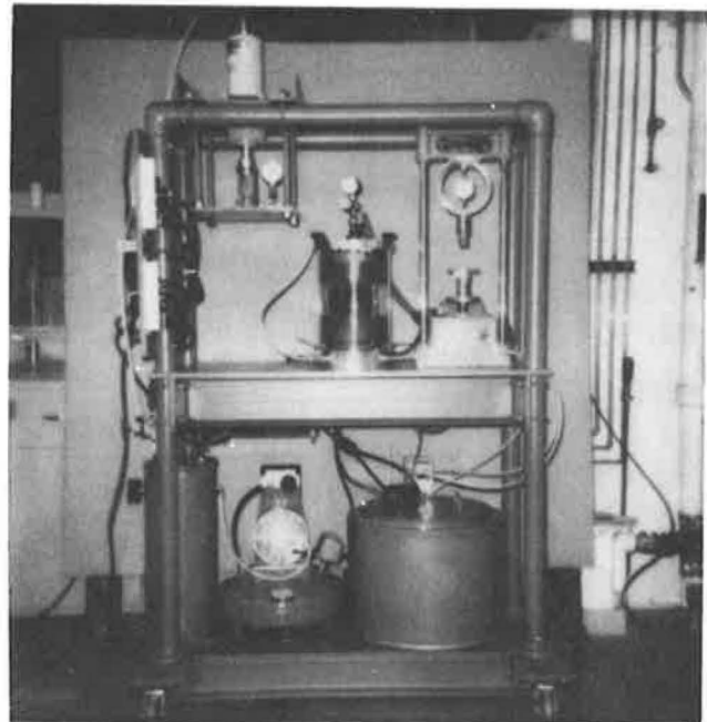
FIGURE 10 Pore water pressure debonding apparatus.
