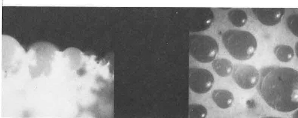
FIGURE 7 Drawdowns and cross section of Systems A, B, C, and D, Sphere 2C (bead rate: 6 lb/100 ft 2 , white). Left , cross section (magnified 100×). Right , top view (magnified 100×).
