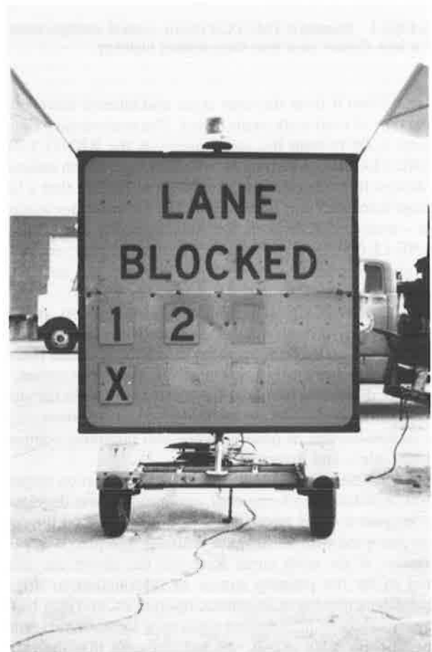
FIGURE 4 The Texas LANE BLOCKED sign.
