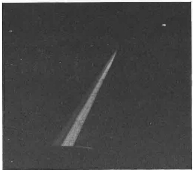
FIGURE 10 Salem, Oregon: large beads in epoxy installed June 1987; large bead edgeline adjacent to standard bead line; Dec. 1987, wet pavement/nighttime.
