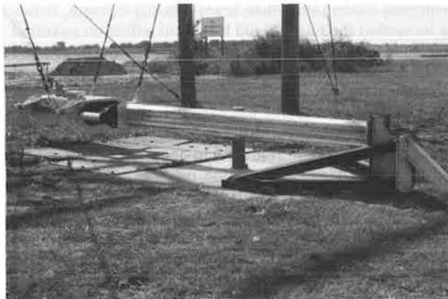
FIGURE 2 Typical pendulum test configuration.
