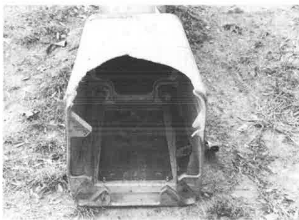
FIGURE 6 Typical transformer-base fracture pattern, bogie impact.
