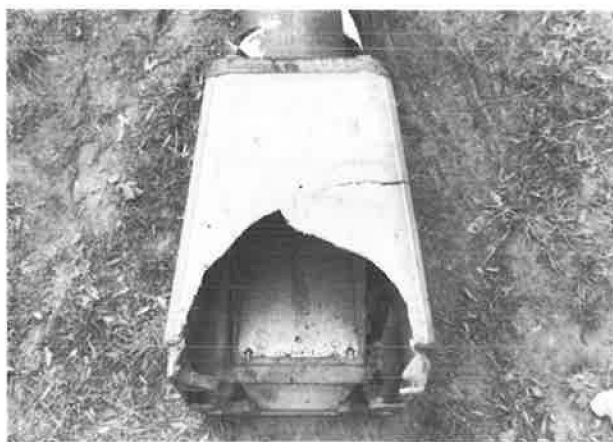
FIGURE 7 Typical transformer-base fracture pattern, automobile impact.
