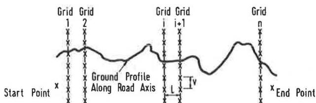
FIGURE 1 Data grid for vertical alignment optimization.
