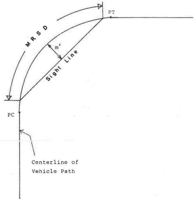
**FIGURE 6** Curve-to-curve sight distance situation.
