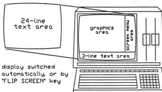
FIGURE 1 Typical single-screen configuration of the AutoCAD system.
