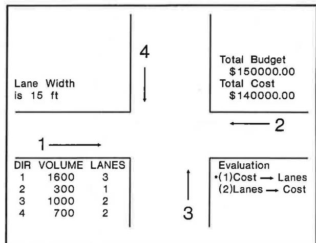
**FIGURE 4** Display screen of the interactive system.
