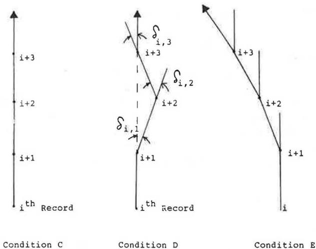
FIGURE 2 Horizontal alignment test conditions.
