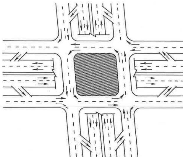
FIGURE 3 Three-level diamond geometrics used in T7F simulation.
