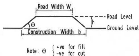
FIGURE 2 Simplified cross section for earth volume computation.
