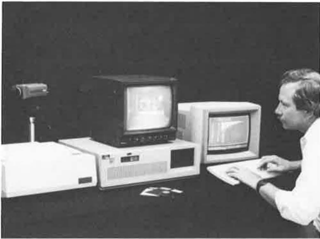
FIGURE 1 Components of the National Research Council Canada luminance and image analysis system known as CapCalc.
