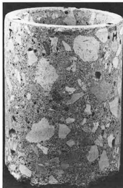
FIGURE 4 A concrete cup before any treatment with salt water. Note the two limestone aggregates at the top just to the left of the letter H.
