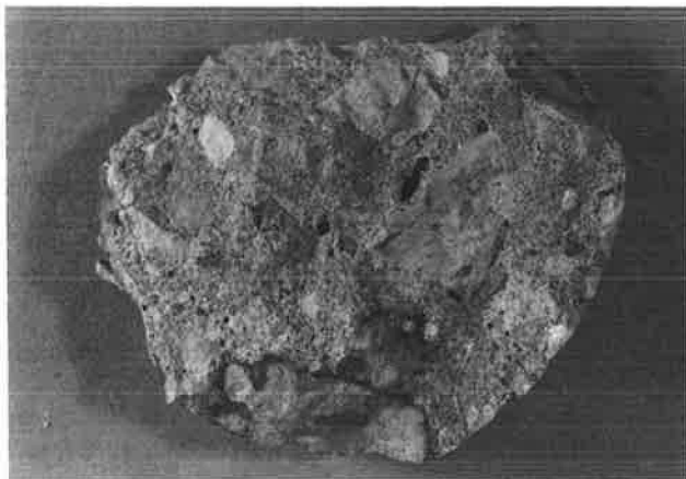
FIGURE 7 PCC containing a deteriorated dolomite aggregate with a dark rim.
