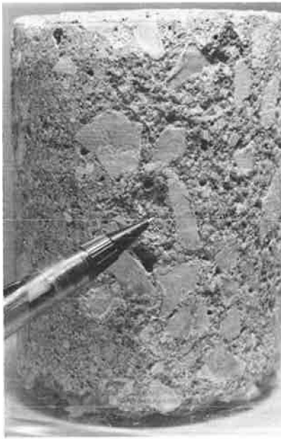
FIGURE 12 The same cup as in Figure 11 after more salt weathering cycles. The bean-shaped aggregate surface has scaled away. The pencil points to where it was. The fragment shown in Figure 8 came from this location.
