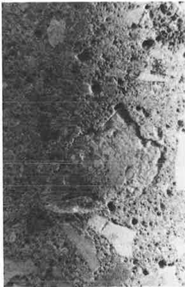
FIGURE 13 A limestone coarse aggregate particle with the entire rim flaked away by salt weathering. This left the aggregate surface depressed relative to the surrounding cement paste. No freeze-thaw was involved. Contrast the aggregate pictured here with those in Figure 9, where the paste was “eaten away” by salt.
