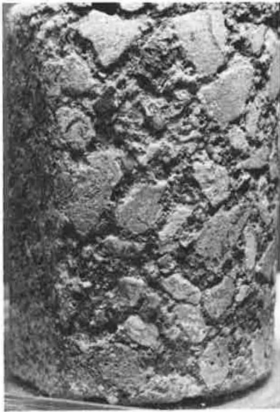
FIGURE 9 A concrete cup that has gone through 12 cycles. Here the aggregates were more durable; the cement paste has weathered away and the limestone aggregates stand out in relief.
