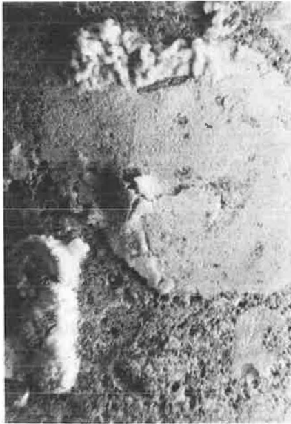
FIGURE 5 The larger of the two aggregates noted in Figure 4. Salt has moved through the aggregate, depositing near its top surface. The salt is also pushing thin flakes from the surface of the aggregate.
