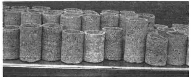
FIGURE 1 A group of concrete cups made by taking two concentric cores such that the cup walls are about ⅜ in. thick and the bottom is at least ½ in. thick.
