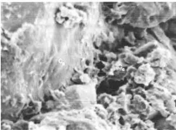
FIGURE 8 Sand mix, 100 percent carbonates, 1 percent Ca(OH) 2 , 30-day soak (3552 ×).
