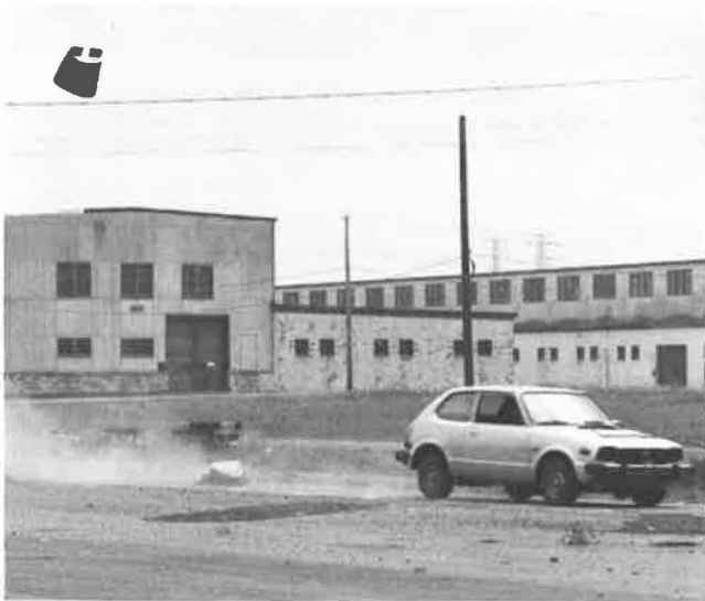
FIGURE 2 Typical impacts with plastic drums ballasted with 50-lb sandbags resulted in drums staying with the front of the car (top), being pushed aside in a brushing impact (center), and two-piece drum being thrown high into the air (bottom).
