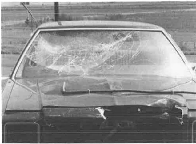
FIGURE 7 A 60-mph impact with a PVC Type III barricade resulted in a shattered windshield.
