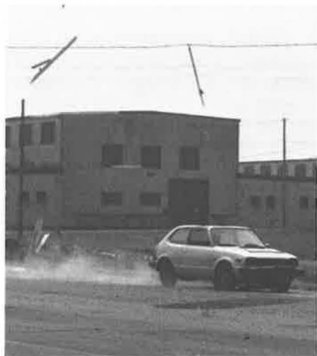
FIGURE 5 A portable low-mounted sign resulted in windshield penetration and debris (top). A tall portable sign resulted in unacceptable debris, although the panel cleared the car (bottom).
