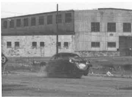
FIGURE 1 An 1,800-lb car impacting a 55-gal steel drum at 60 mph resulted in loss of vehicle control.
