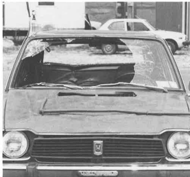
FIGURE 3 A 42-lb concrete-block ballast placed on a drum resulted in unacceptable intrusion into the passenger compartment.
