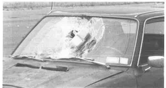
FIGURE 4 Attaching warning light to channelizing drums resulted in lights being thrown on impact and drums flying over the vehicle (top), with varying degrees of windshield damage (bottom).
