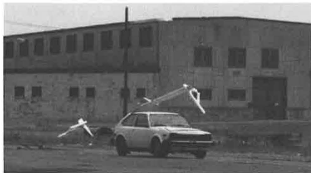
FIGURE 6 Collision with a Type I barricade resulted in unacceptable debris.
