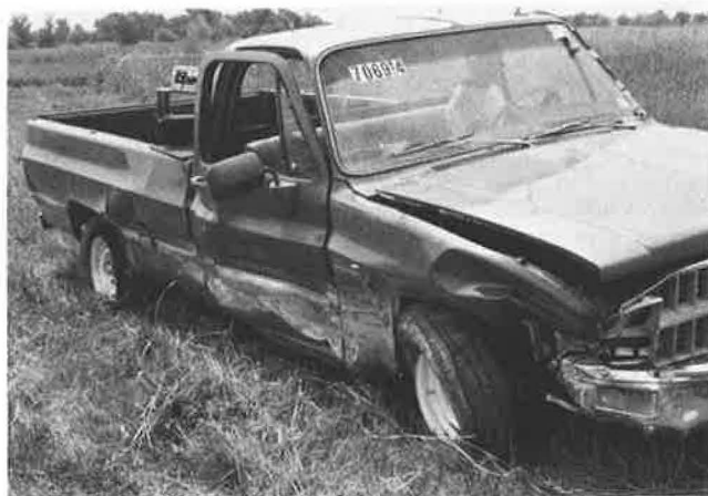
FIGURE 25 Damage to vehicle in Test 7069-4 (5,440 lb, 65.4 mph, 20.4 degrees).
