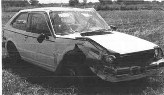
FIGURE 22 Damage to vehicle in Test 7069-3 (1,800 lb, 60.1 mph, 21.4 degrees).
