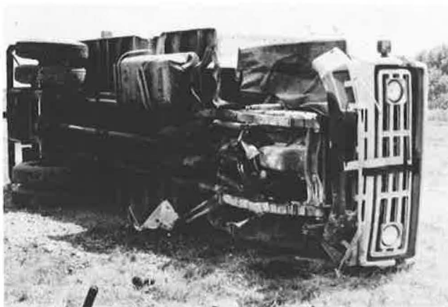
FIGURE 36 Damage to vehicle in Test 7069-12 (18,000 lb, 51.6 mph, 15.5 degrees).
