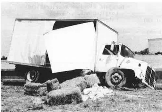
FIGURE 8 Photograph of vehicle after Test 7069-15 (18,000 lb, 50.8 mph, 15.1 degrees).
