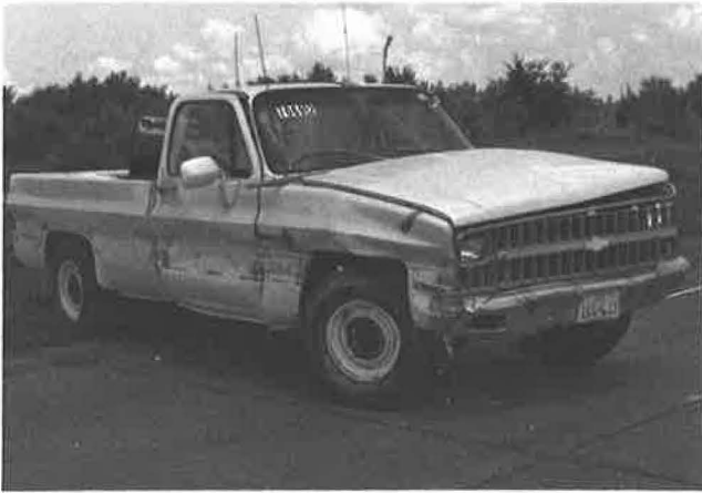
FIGURE 5 Damage to vehicle in Test 7069-2 (5,450 lb, 63.6 mph, 19.2 degrees).
