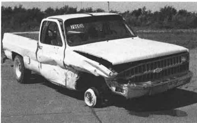
FIGURE 15 Vehicle after Test 7069-6 (5,400 lb, 59.7 mph, 20.2 degrees).
