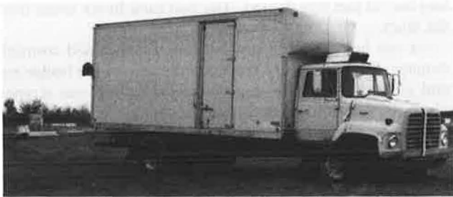
FIGURE 28 Vehicle after Test 7069-11 (18,000 lb, 52.1 mph, 14.8 degrees).
