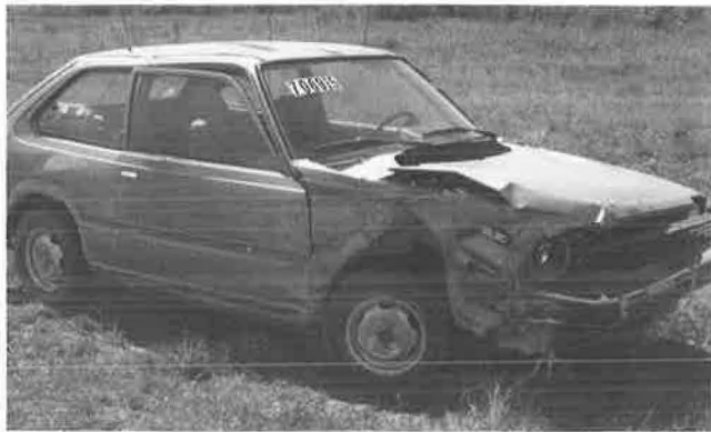
FIGURE 12 Vehicle after Test 7069-5 (1,800 lb, 60.5 mph, 21.0 degrees).
