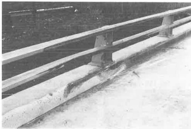
FIGURE 4 Barrier and vehicle damage after Test 0368-2.
