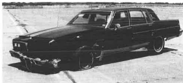
FIGURE 9 Barrier and vehicle damage after Test 0382-2.
