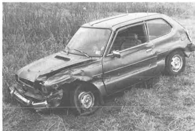
FIGURE 2 Barrier and vehicle damage after Test 0368-1.
