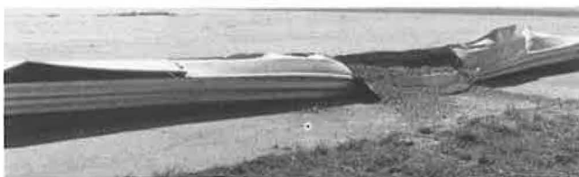
FIGURE 4 MK-9 barrier after Test 7091-2.
