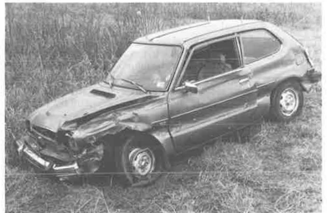
FIGURE 2 Barrier and vehicle damage after Test 0368-1.
