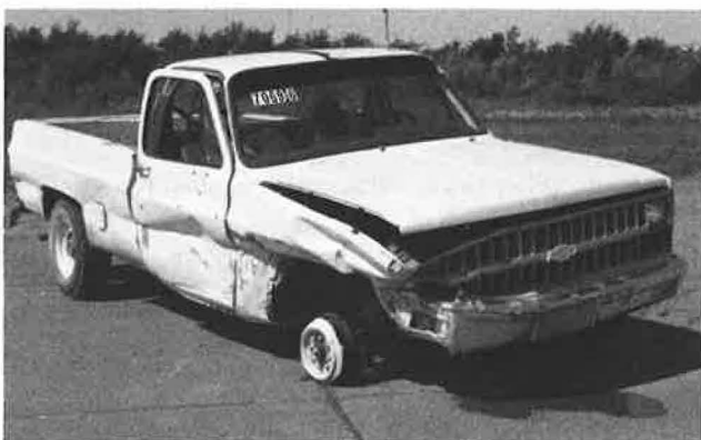
FIGURE 15 Vehicle after Test 7069-6 (5,400 lb, 59.7 mph, 20.2 degrees).
