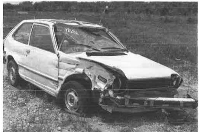
FIGURE 3 Vehicle after Test 7069-1 (1,795 lb, 58.7 mph, 20.0 degrees).
