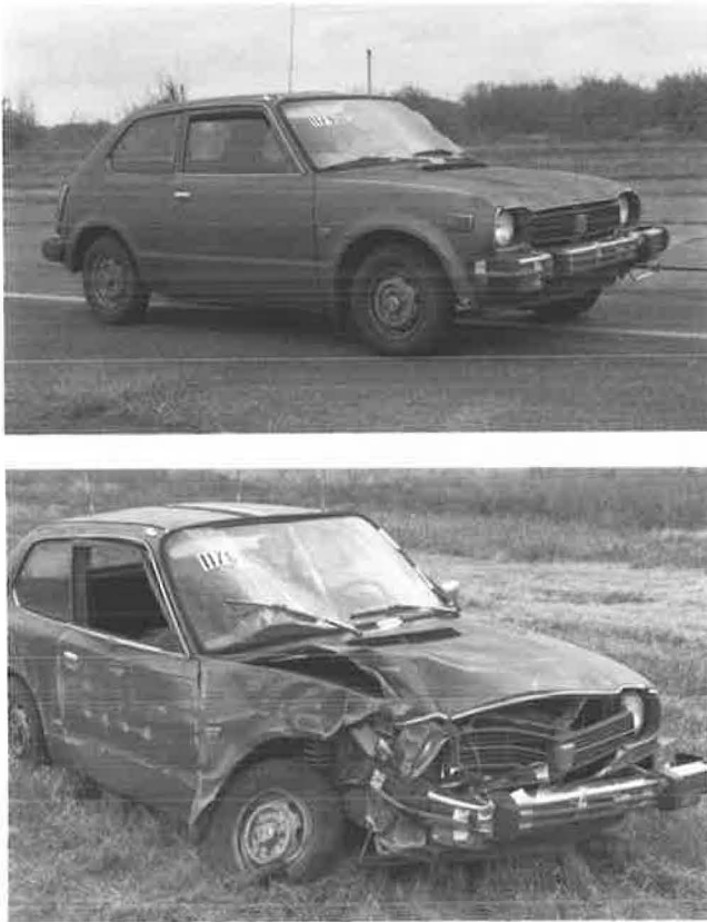
FIGURE 5 Vehicle before and after Test 1179-1.
