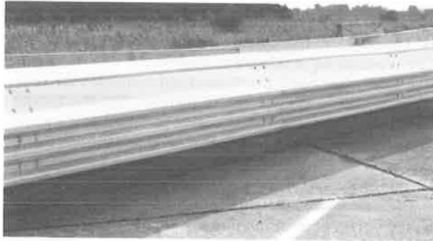
FIGURE 10 IBC MK-7 barrier test installation.
