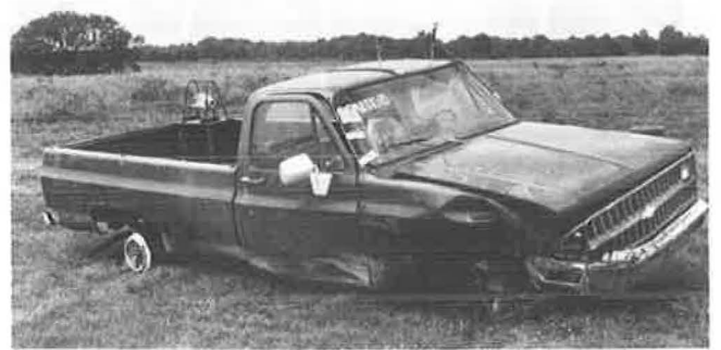
FIGURE 33 Damage to vehicle in Test 7069-14 (5,390 lb, 57.7 mph, 20.6 degrees).
