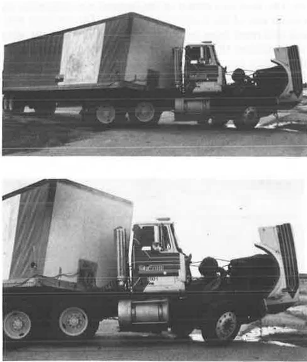
FIGURE 14 Tractor-trailer after Test 7132-1.
