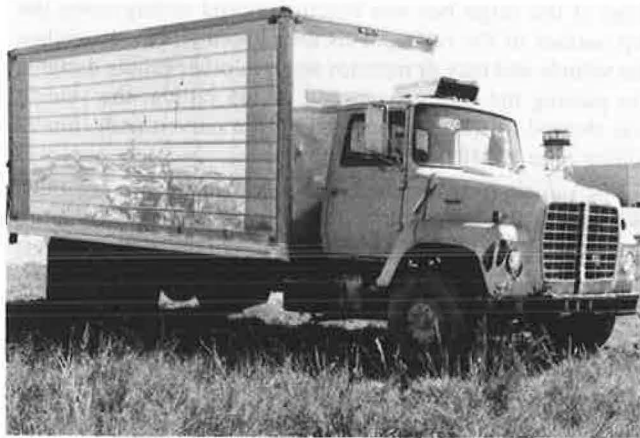
FIGURE 18 Damage to vehicle in Test 7069-16 (18,000 lb, 50 mph, 14 degrees) after being uprighted.
