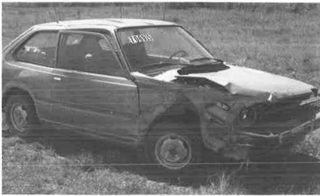
FIGURE 12 Vehicle after Test 7069-5 (1,800 lb, 60.5 mph, 21.0 degrees).
