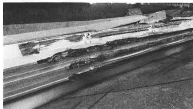
FIGURE 13 IBC MK-7 barrier after Test 7132-1.
