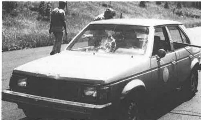
FIGURE 15 Preliminary crash test windshield damage from 41-in.-clearance aluminum sign.
