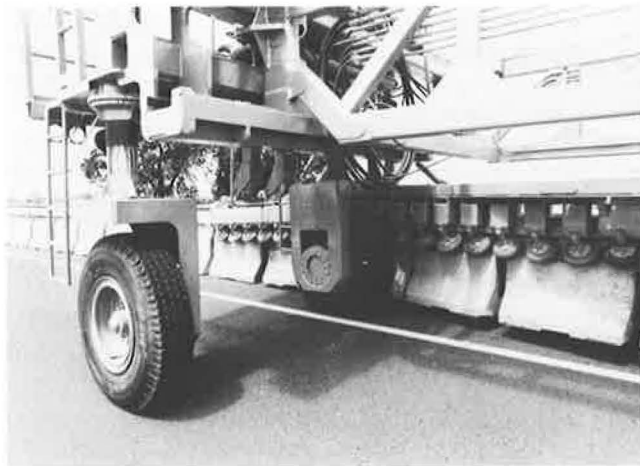
FIGURE 3 Barrier is lifted by conveyor wheels under the MCB flange.
