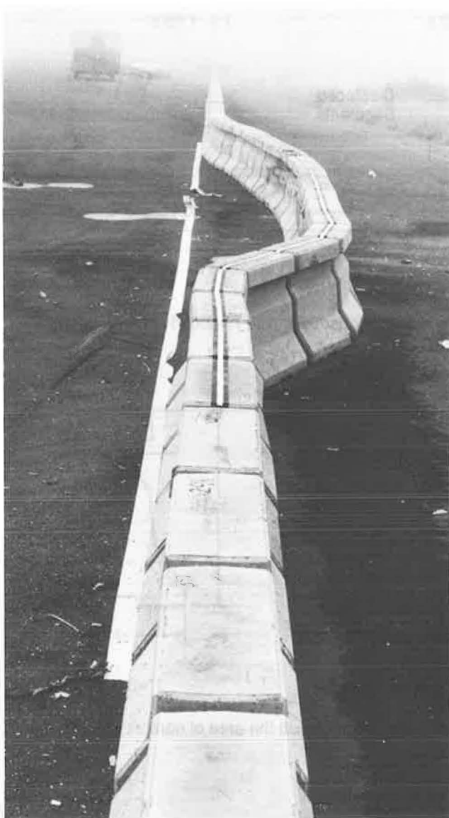
FIGURE 8 Deflected barrier after impact, Test 443.
