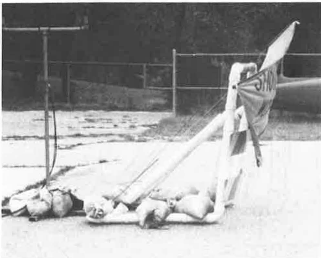
FIGURE 3 Phase 2 wind test with 1-ft-clearance vinyl sign at 69 mph.
