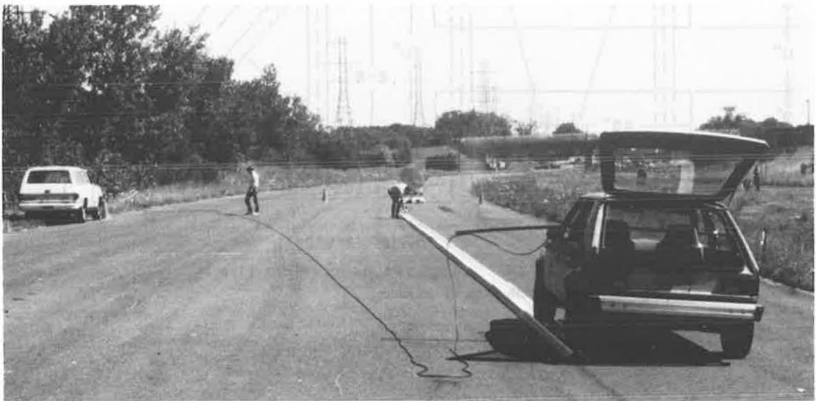
FIGURE 12 Preliminary crash test vehicle guidance system.
