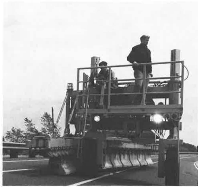
FIGURE 20 Transfer vehicle carrying barrier.
