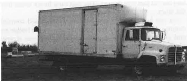
FIGURE 28 Vehicle after Test 7069-11 (18,000 lb, 52.1 mph, 14.8 degrees).
