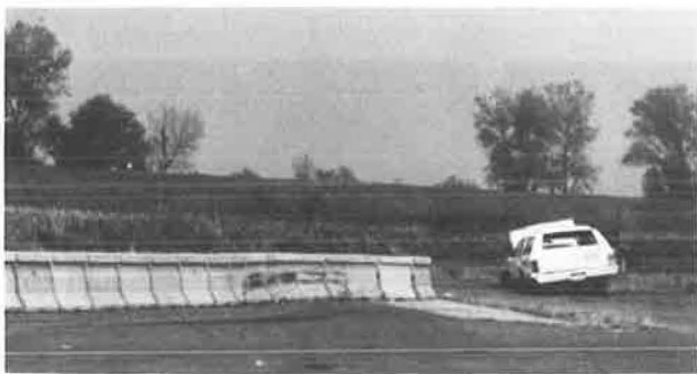
FIGURE 7 Car and barrier after impact, Test 443.
