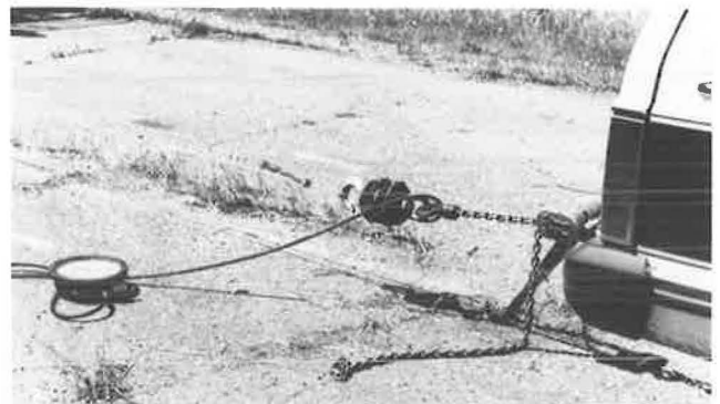
FIGURE 23 Tensioning the tether cable.
