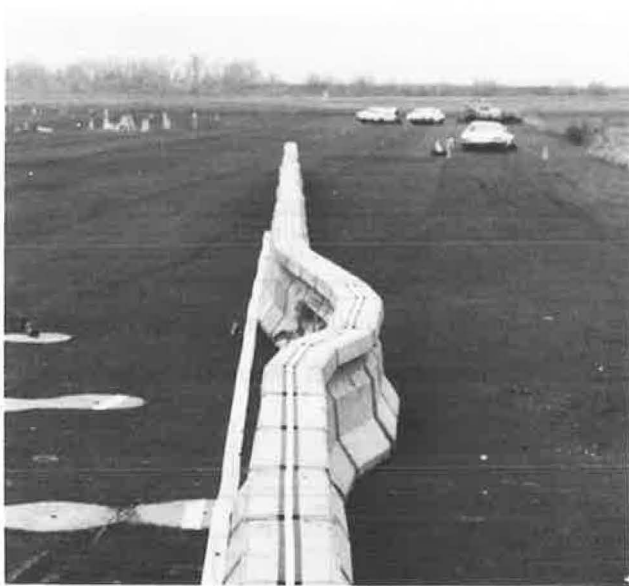
FIGURE 11 Deflected barrier after impact, Test 444.
