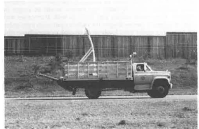
FIGURE 2 Phase 1 wind test with 7-ft-clearance vinyl sign at 45 mph.
