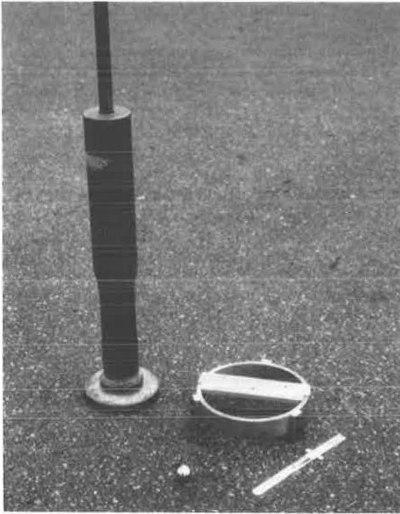
FIGURE 5 Equipment required for Ball Penetration Test.
