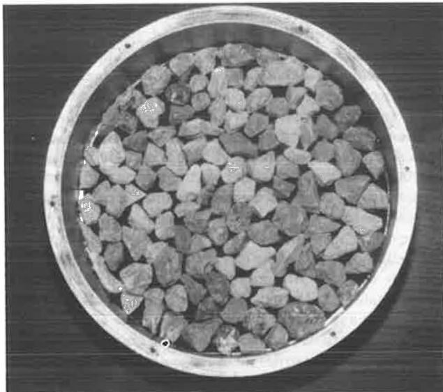
FIGURE 1 Packing of stone in modified tray.
