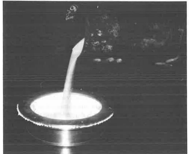
FIGURE 3 Pouring density sand into modified tray.
