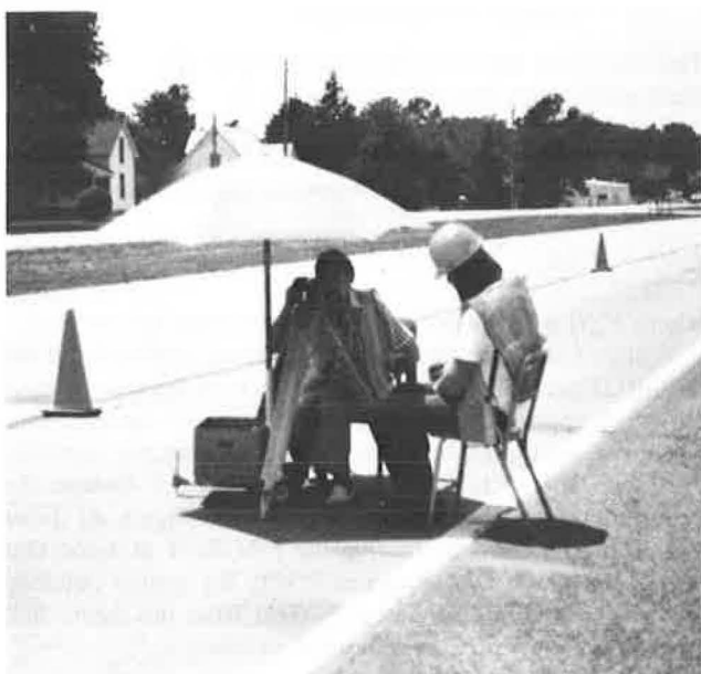
FIGURE 3 The instrument used to collect the rod and level data.
