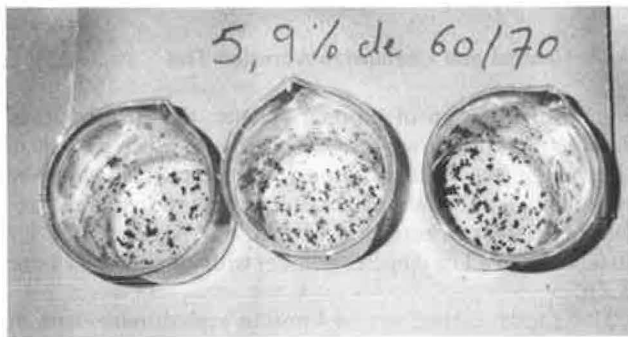
FIGURE 3 View of the glass receivers after the Schellenberger drainage test. (Porous asphalt with 5.9 percent bitumen and 0.3 percent fibers.)
