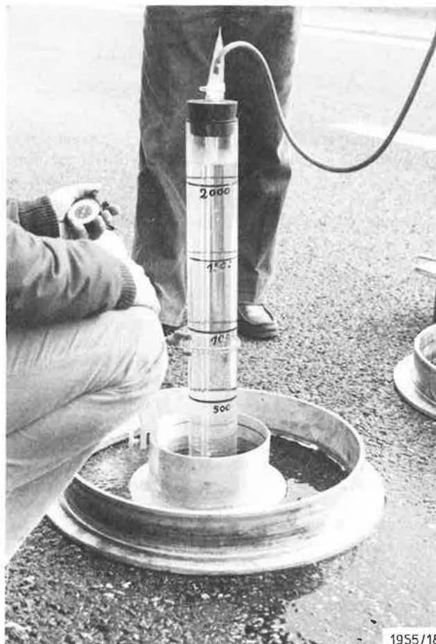
FIGURE 8 In situ measurement of the draining capacity of porous asphalt.
