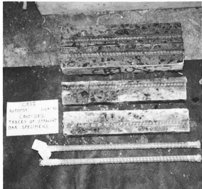
FIGURE 12 Rebars after completion of autopsy of a slab representing Variable 10.
