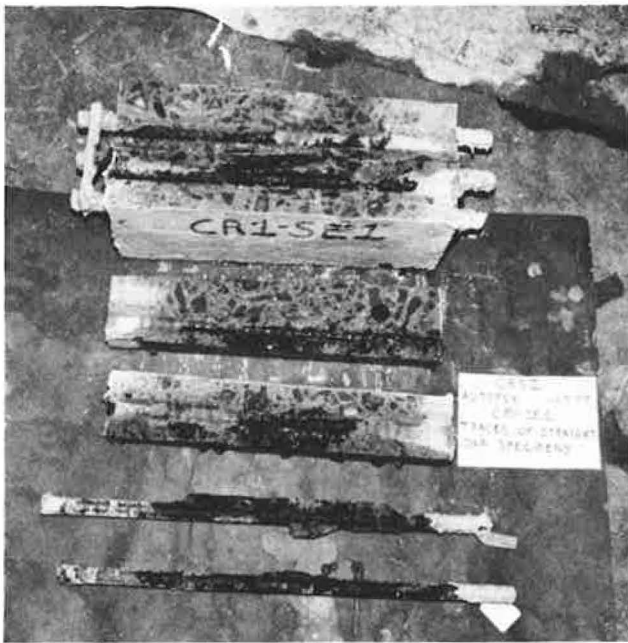
FIGURE 11 Rebars after completion of autopsy of a slab representing black bar controls.
