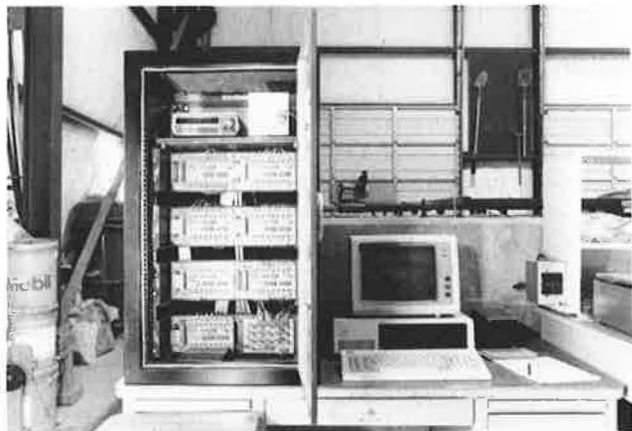
FIGURE 8 The computer and the cabinet containing the multiplexing cards.
