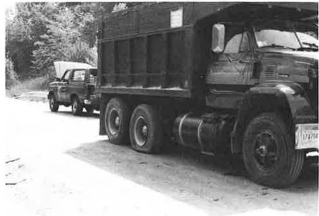
FIGURE 4 Application of live load (note flat tires on central axle to shift weight to rear axle).
